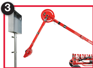
Align with conduit, properly adjust booms
