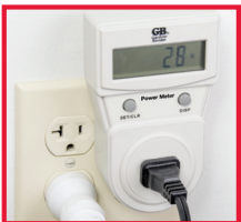
Measure energy consumption for cost planning
